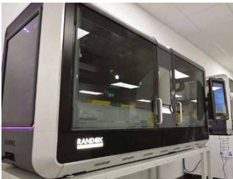
Figure 6(2): The Randox Discovery, a fully automated, benchtop PCR system
